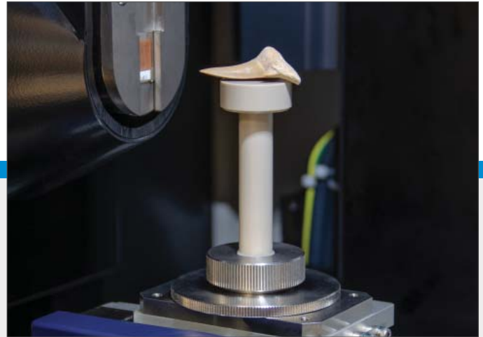
Small sample stage with shark tooth and view of X-ray source
